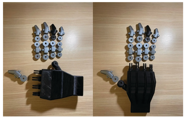
Fig. 8. 3D printed hand prosthesis – before assembly
