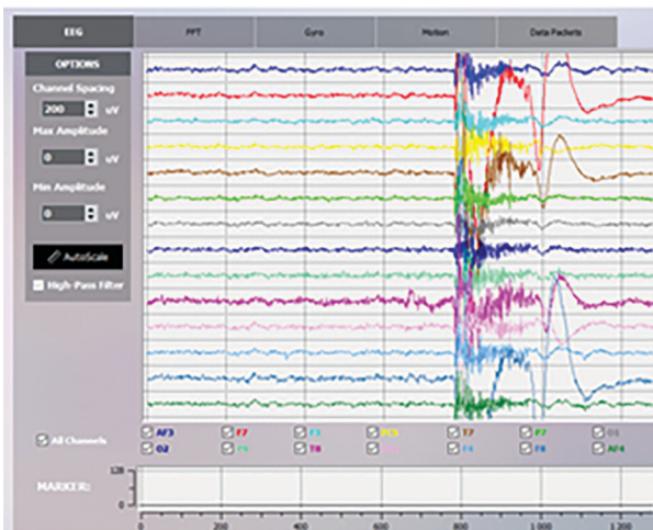
Fig. 13. Artifact – EEG signal during clenching teeth
