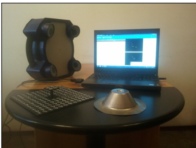
Fig. 6. Photography of movable strain analyzer AutoGrid in compact version used at industrial trials
