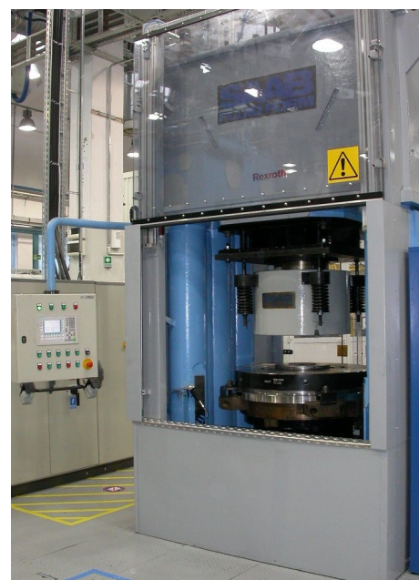
Fig. 3. Photograph of industrial hydraulic stamping machine for forming with the use of liquid
