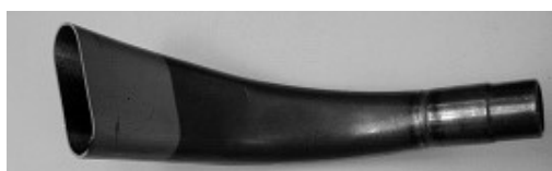
Fig. 1. A pressed element made of nickel superalloy by stamping and joining
