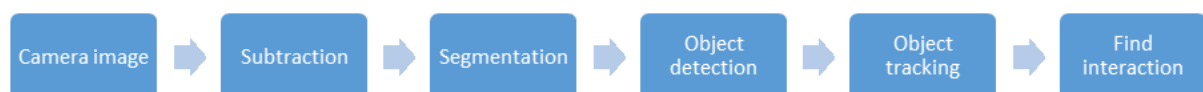
Figure 1. Logical steps of the implemented algorithm. Adapted from: “Shopper analytics: A customer activity recognition system using a distributed RGB-D camera network” by D. Liciotti et al. Copyright 2014 by Springer.
