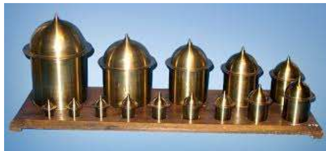
Fig. 3. Tubular Helmholtz resonator [26].
