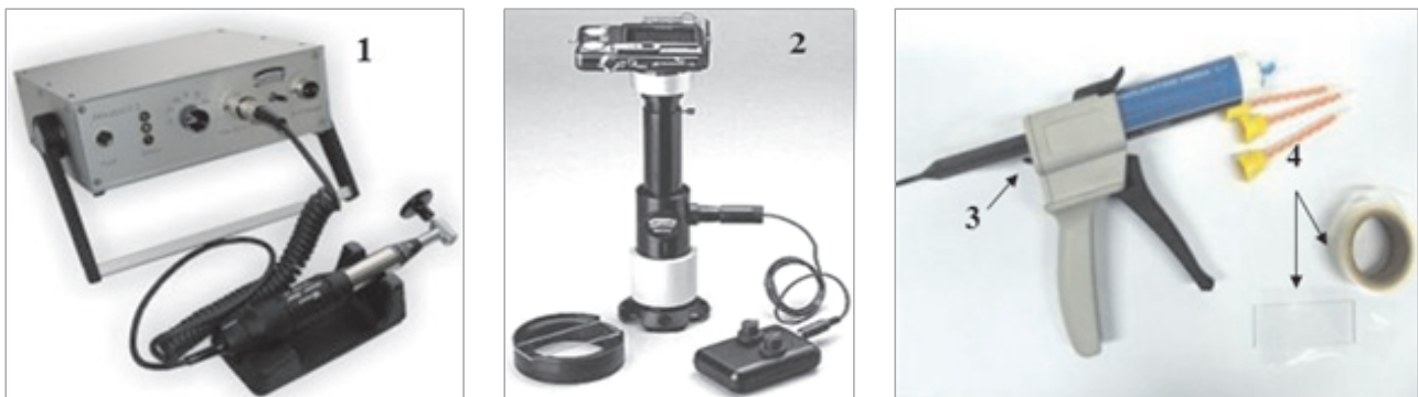
Fig. 7. Equipment for non-destructive metallography: 1) grinding-and-polishing machine Akkupol, 2) portable light field microscope TCM, 3) press for «liquid» replicas, 4) replicas
