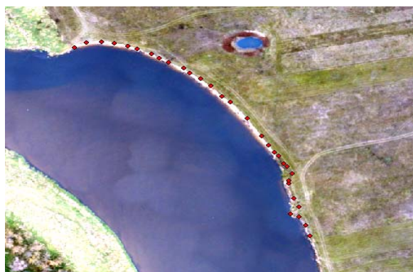
Fig. 2. Visualization of points which had been measured using the GPS RTN technique; source: own elaboration
