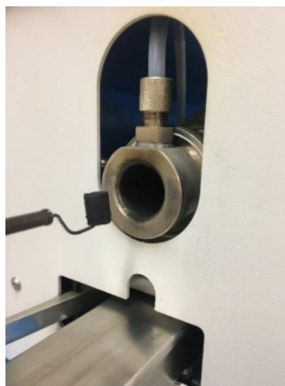
Fig. 1. View of prepared coal sample mounted on a thermocouple prior to insertion into the furnace.
