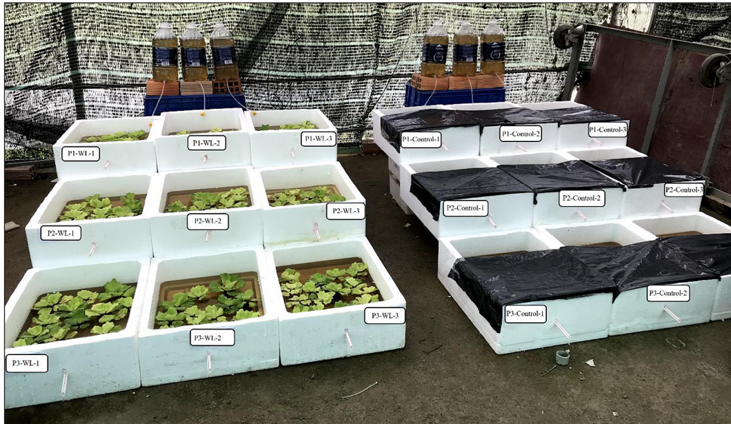
Figure 1. Experimental system [terraced styrofoam containers designed as pond 1(P1), pond 2(P2) and pond 3(P3)]
