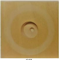
PUR OIL Figure 1. Traces on surface finish after resistance to abrasion testing.
