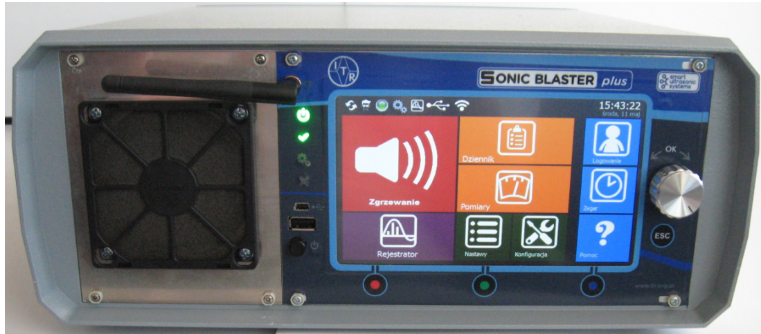
Fig. 9. Generator front panel displaying main menu.
