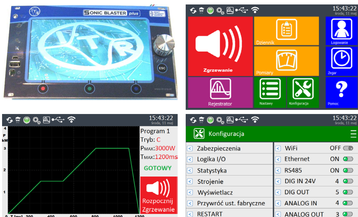
Fig. 8. Control panel photo (top left), Main menu (top right), Welding curve menu (bottom left), Configuration menu (bottom right).
