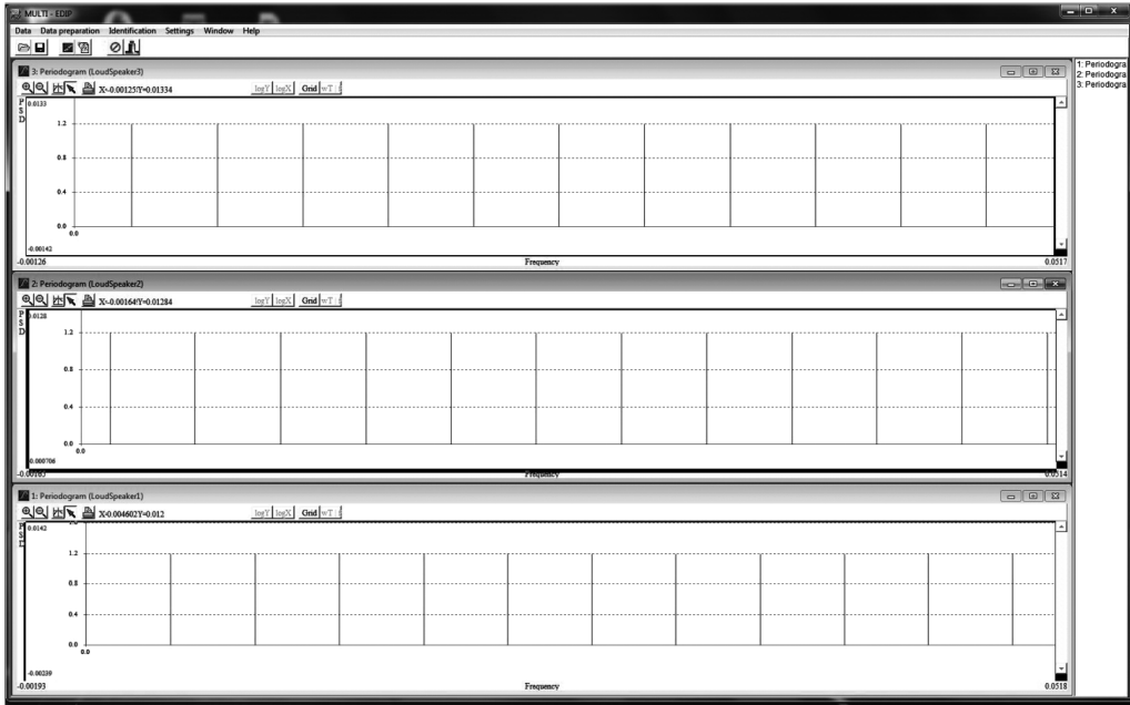
Figure 3. Power spectral densities calculated for three elements of input signal - a zoom in frequency.
