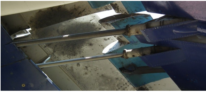
Fig. 1. Actuators with screw gear controlling the positioning of the flaps in the IL-76 transport aircraft
