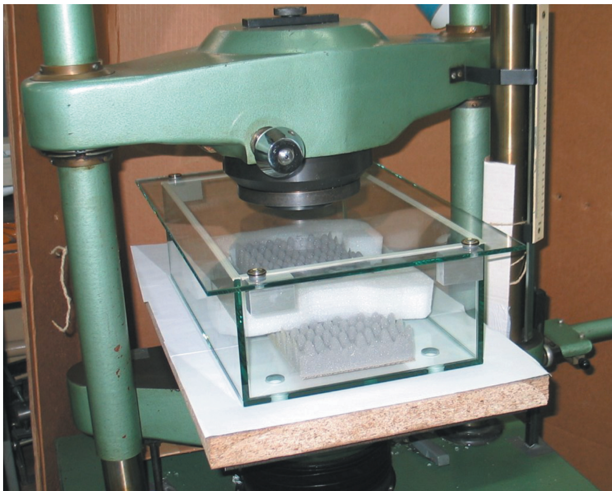
Fig. 6. Strength test of display case – closed case with protective glazing
