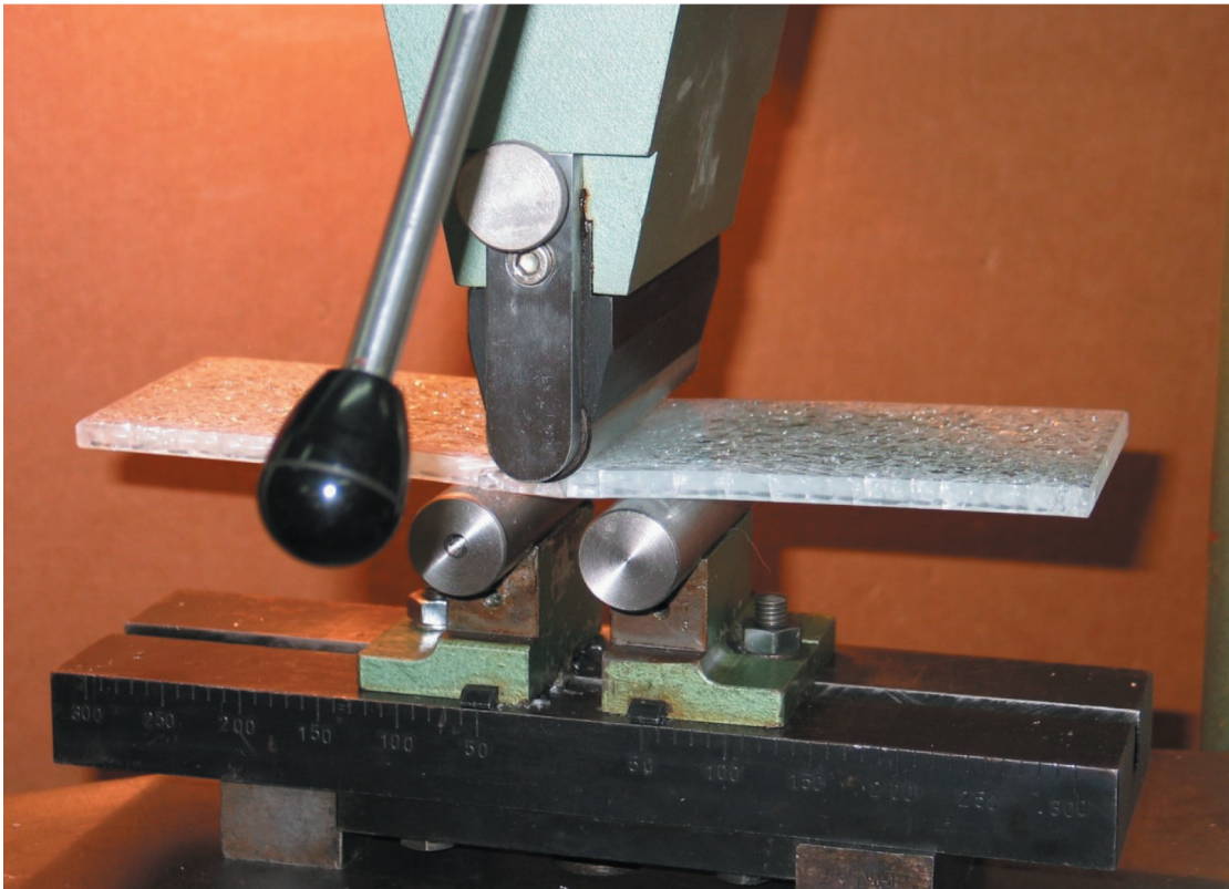
Fig. 2. Studies on transversal bending strength for 8 mm-thick glass samples with polished edge and 0.22 mm security film
