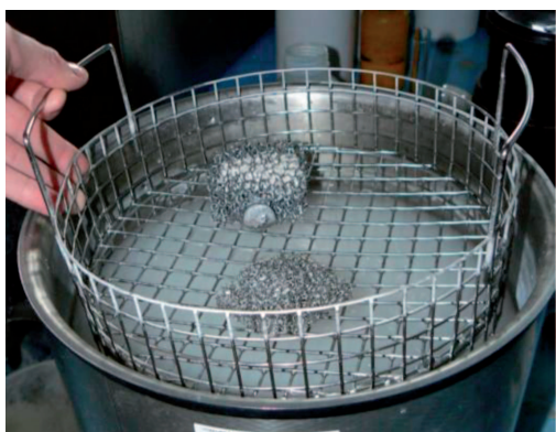
Fig. 6. Cleaning of metallic filters in ultrasonic bath
