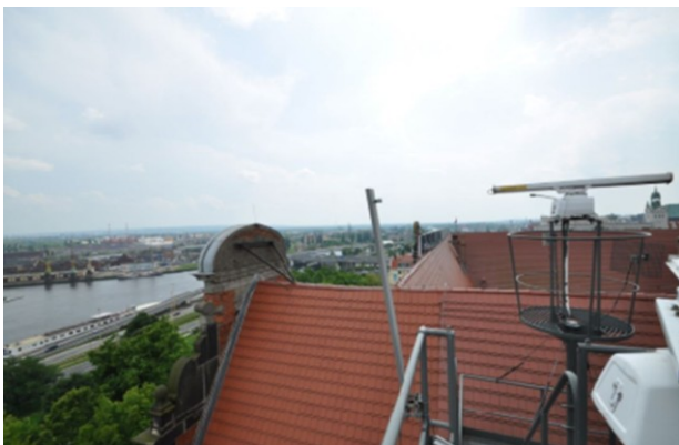
Fig. 6. The radar sensor and an attic that is the source of blind sector
