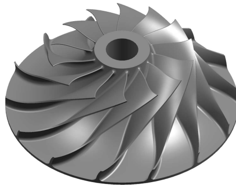
Figure 13: The impeller geometry described with the Gauss curvature
