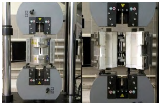
Fig. 1. Furnace for high-temperature testing.
