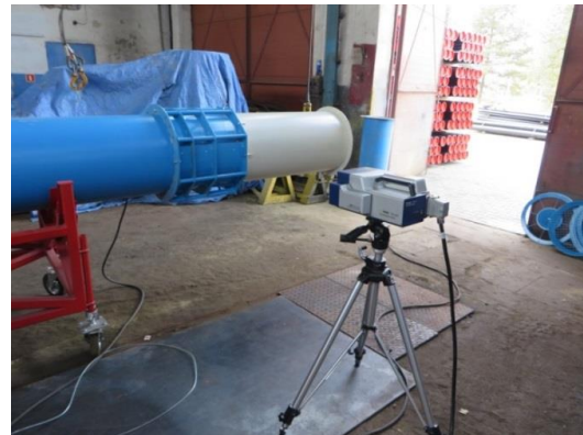
Fig. 2. Laser Doppler Vibrometer during measurements of casing vibrations
