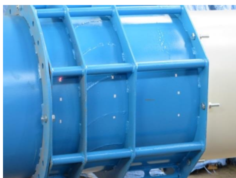
Fig. 1. Casing of WL-S 500 axial fan prepared to experimental measurements with use of LDV
