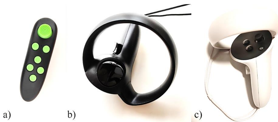
Fig. 3. Examples of different types of a) simple remote controller, b) oculus rift and c) oculus quest 2 controllers.
