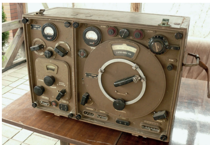
Fig. 5. Radio station N1, in a version produced by the Germans as F1. A frontal plate of the radio station consisted of 2 panels. The wider panel was a transmitter. The narrower panel – which can be seen on the left side – constituted a receiver of this radio station – note AN Source: Photo and instruction made available by inż. Bogdan Szkuclarek SP3LD – Polish amateur radio operator and collector of communication equipment.
