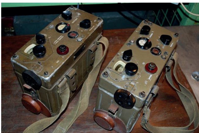
Fig. 7. Receiver of the radio station N2 produced by the Germans as AQ 2 during the war Source: Photo and instruction made available by inż. Bogdan Szkudlarek SP3LD – Polish amateur radio operator and collector of communication equipment.
