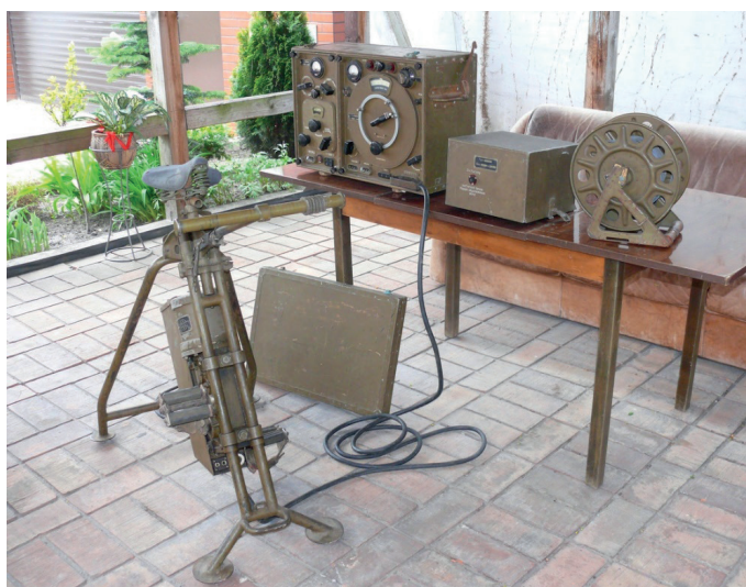
Fig. 6. Radio station N1 in a German version together with a pedal-supply system Source: Photo made available by inż. Bogdan Szkuclarek SP3LD.
