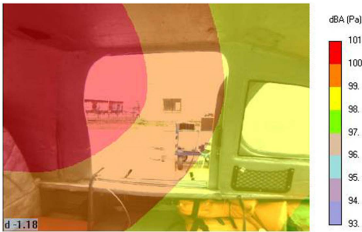
Fig. 6. The distribution of the noise sources on the left wall of the cabin – the door opened. [S. Cieślak, 2016]
