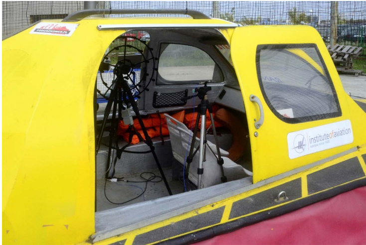
Fig. 2. Hovercraft PRC-600M while measuring a noise level in the cabin. [W. Krzymień, 2016]
