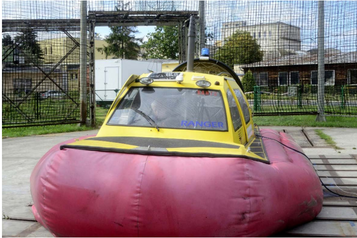
Fig. 1. Hovercraft PRC-600M during noise level tests. [W. Krzymieć, 2016].
