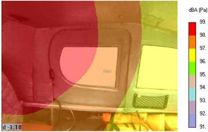
Fig. 5. The distribution of the noise sources on the left wall of the cabin – the door closed. [S. Cieślak, 2016]
