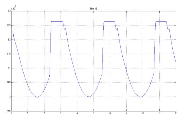
Fig. 5. The time progress of the pressure difference (Pa) between the pump input and output
