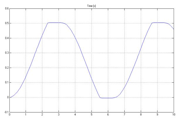
Fig. 2. The time progress of the relative hydraulic cylinder piston rod distance (m)
