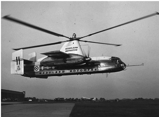
Fig. 9. Fairey Rotodyne as an example of gyrodyne [14]
