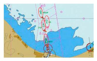
Figure 3. Proposed ship domain on VTS operator screen
