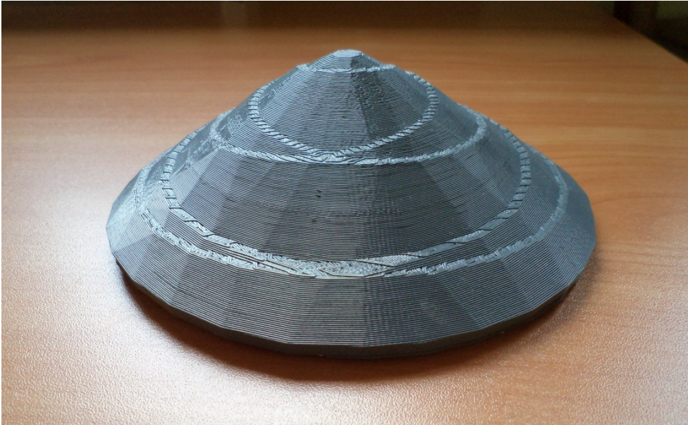
Fig. 1. Model of the Piłsudski Mound obtained in the process of 3D printing in scale of 1:800. Printing time – eight hours, on the slopes of the mound you can see paths leading to the top, the measuring of the 270 points did not provide the smoothness of the model, as indicated by visible edges at the junction of triangles covering the surface
