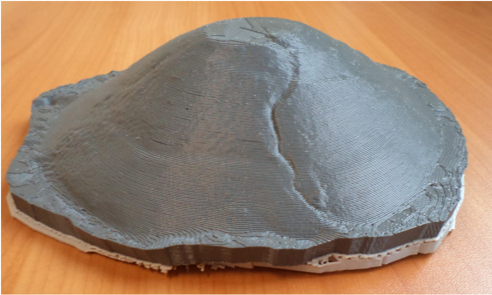
Fig. 3. The Krakus Mound model, scale 1:500. Printing time – six hours, the method of laser scanning and of point cloud elaboration provides the high accuracy of reproducing details, on the slope of the mound you can see paths and local elements of micro-relief of the terrain
