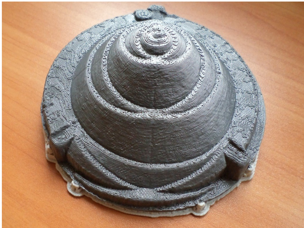
Fig. 4. Model of the Kościuszko Mound, scale 1:800. Printing time – seven hours, high accuracy of reproducing allowed the accurate representation of the path leading to the top and the fort fragments; the thickness of the elementary layer of 3D printing is approximately 0.2 mm
