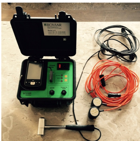
Fig. 2. Ultrasonic instrument Boviari with technical data
