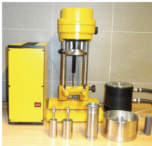
Fig. 1. Viscometer Rheotest RN4.1 with the equipment
