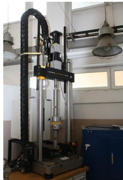
Fig. 1. Static and dynamic testing machine Instron 8872.
