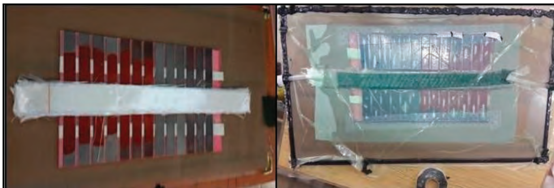
Fig. 3. Specimen fabrication with vacuum bagging technique
