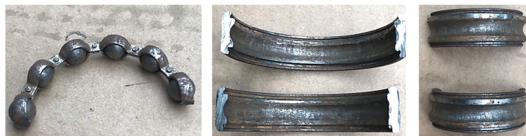
Fig. 3. Wear of the main bearing elements: rolling elements, outer and inner raceways
