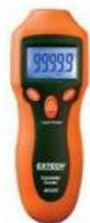
Measure the speed of rotation of the active crawler without contact with the Extech - 461920, measured at idling.
