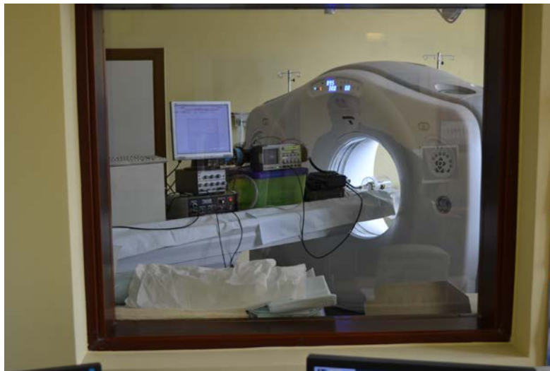
Fig. 4. CT setup for elastic properties measurements of the LV model.
