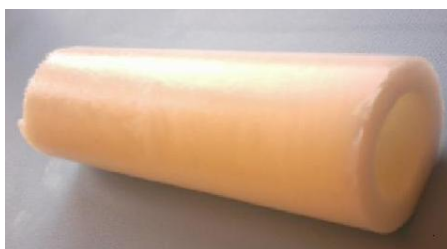
Fig. 2. The LV phantoms: a) – normal, b) with stiffened wall imitating the myocardial infarction.
