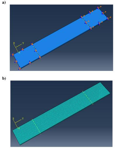
Fig. 3. Numerical model: a) Boundary conditions, b) Mesh [source: own research]
