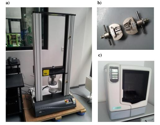
Fig. 2. Test stand: a) Machine Instron 3369, b) Manual jaws Instron 50 kN, c) 3D printer uPrint SE [source: own research]
