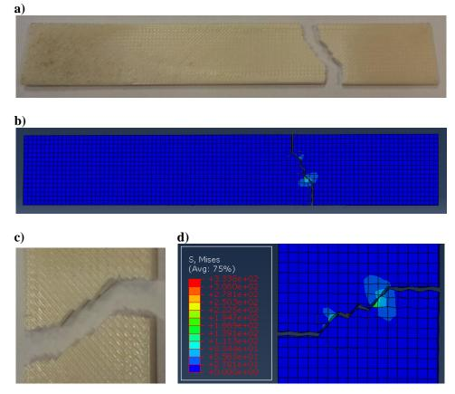
Fig. 4. The comparative results of numerical analysis and experimental study:
