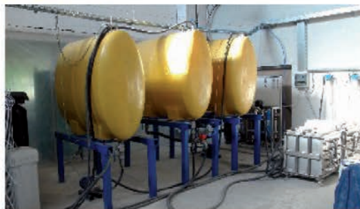
Fig. 7. A prototype of a technological line for processing decorticated flax fibre: a) view of the prototype of the technological line, b) – reactor, c) – unrolling module, d) – degumming module, e) – wringing modules, f) – water production and purification
