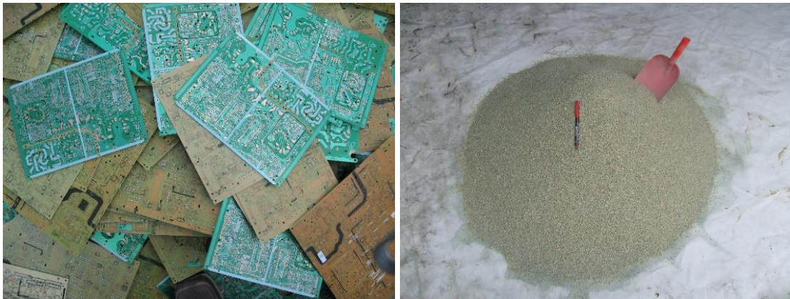
Fig. 2. Scrap TV boards (STVBs) (left) and size-reduced STVBs ( -3.35 mm) (right)
