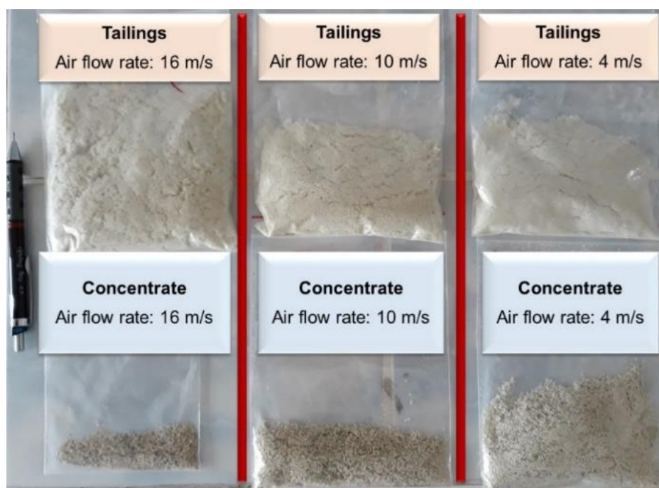
Fig. 4. Photos of the products (concentrate and tailings) obtained from zig-zag air separation tests of STVBs under different flow rates of air (4-16 m/s)
