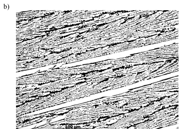
Fig. 7. Microstructure of a) eutectic, b) hypereutectic structure areas - samples after solidifying was frozen (immediately taken off the cooler), v=83.3 \mu\text{m/s} , G=33.5 \text{ K/mm}
