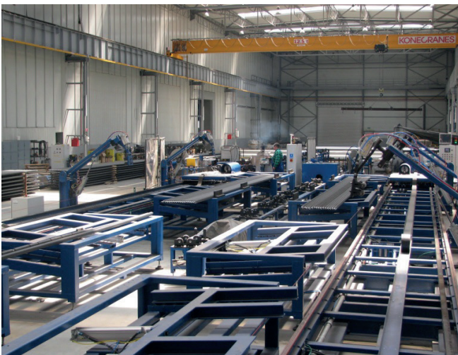
Fig. 2. General view of the station for the welding of finned tubes in the company Energoinstal SA
