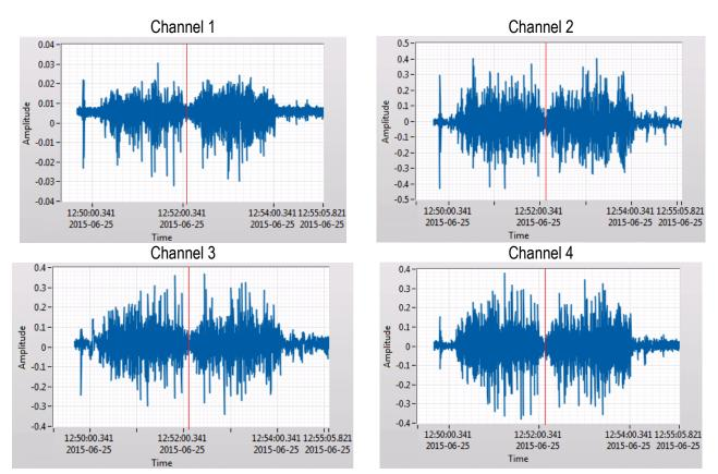
Fig. 4. The measured profile of excitations (empty wagon and max. speed 10 km/h)
