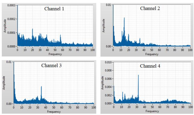
Fig. 5. An example of results of measured signal FFT analysis
