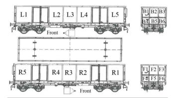
Fig. 1. Designation of EAOS 1415 A2 and A3 wagon's elements, where symbols denotes: L – the left side, R – the right side, F – the front, B – the back of the wagon
