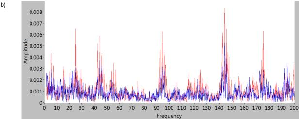
Fig. 9. Results of the FFT analysis of measured signals juxtaposed for the system witch (the blue line) and without (the red line) composite panels for channel 1 (a) and channel 2 (b)
