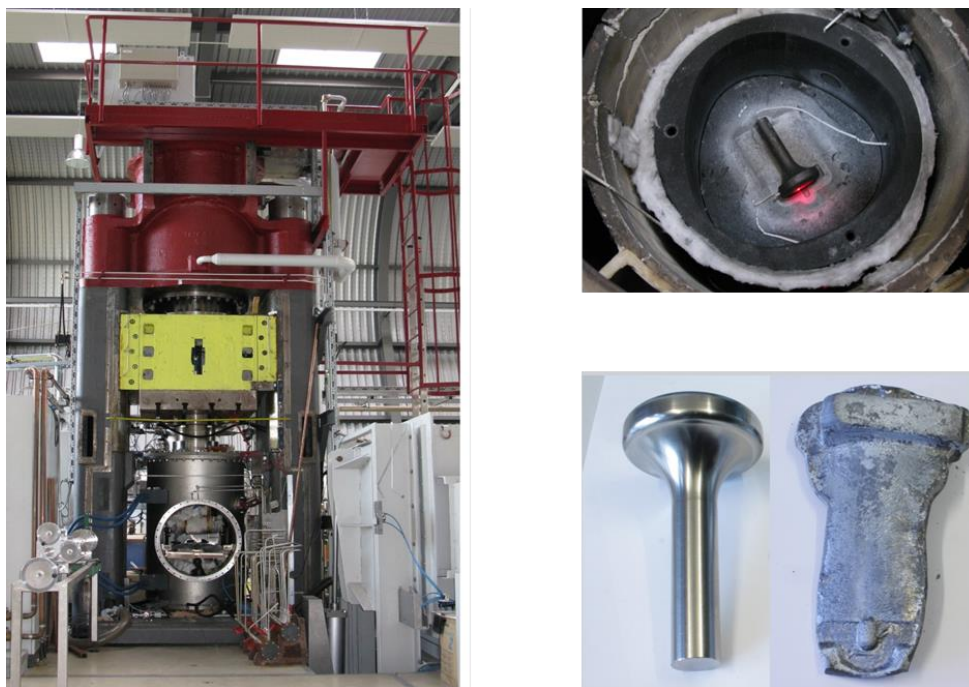
Fig. 1. (Left) 1700 ton isothermal forging press. (Top right) Lower die with part in vacuum chamber. (Bottom right) TiAl workpiece and forged turbine blade
