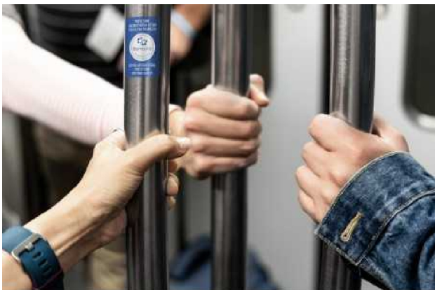
Fig. 8. Wagon handrails covered with the antibacterial film [26]
