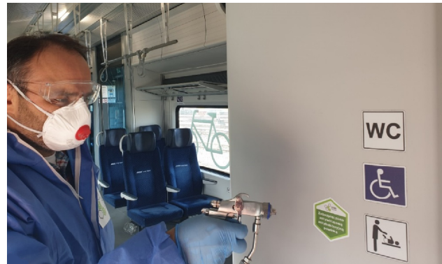
Fig. 6. Applying an antimicrobial coating to wagon walls [12]
