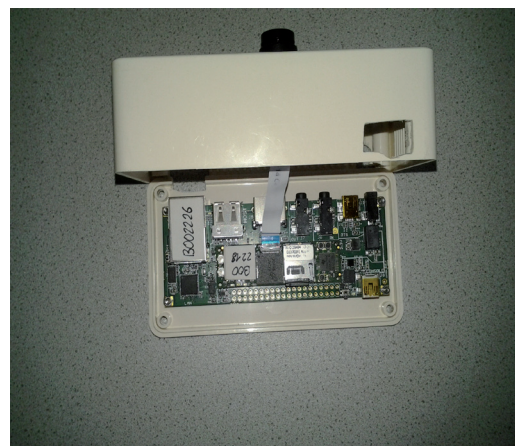
Fig. 7. Development setup for the Gumstix computer with Tobi expansion board and Caspa camera
