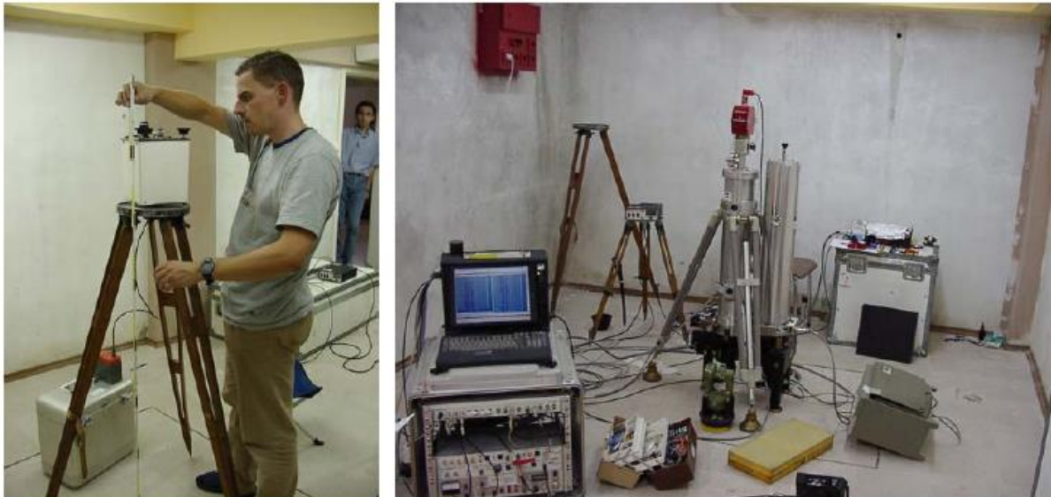
Fig. 4.3.10.3. Measurement of the gravity gradient and the absolute value in Varna
