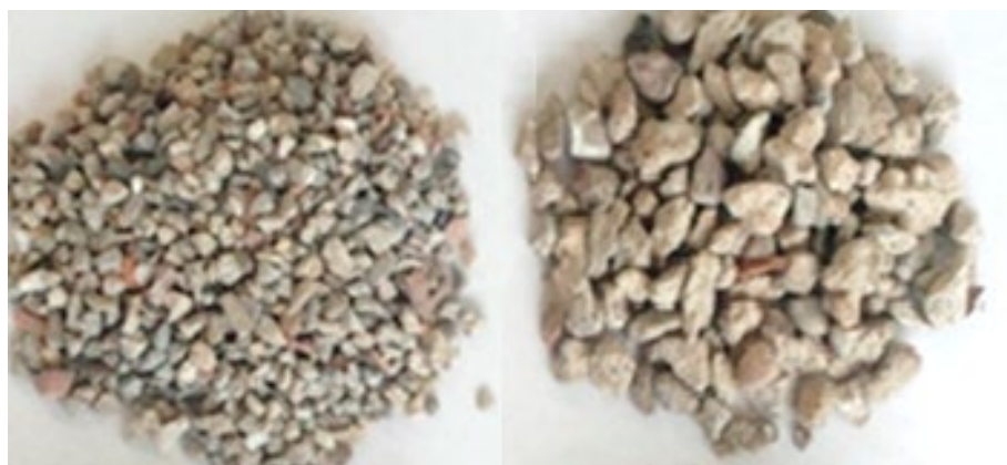
Figure 5. Aggregate from concrete recycling
