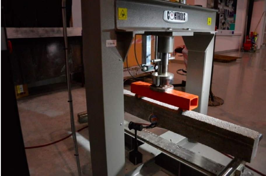
Figure 10. Test stand for reinforced concrete model beams
