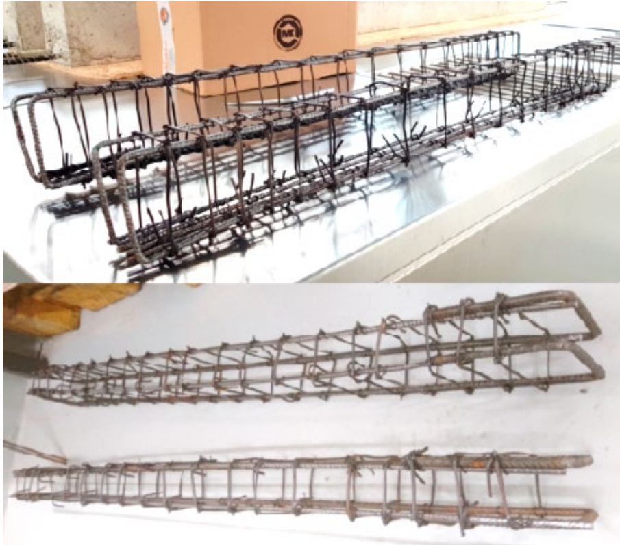
Figure 7. Reinforcing frames of reinforced concrete beams – top basalt rebars, bottom steel rebars
