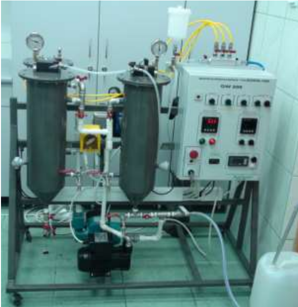
Fig. 2. Reactor GW 200 for production of Biodiesel FAME (FAEE)
