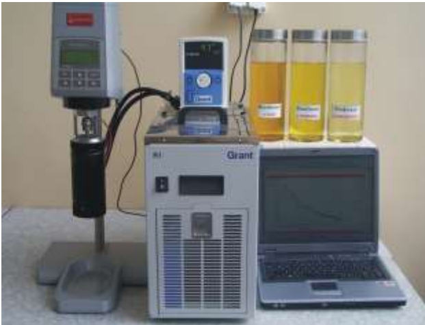
Fig. 3. The researchers post was furnished with a reometer and tub thermostats
