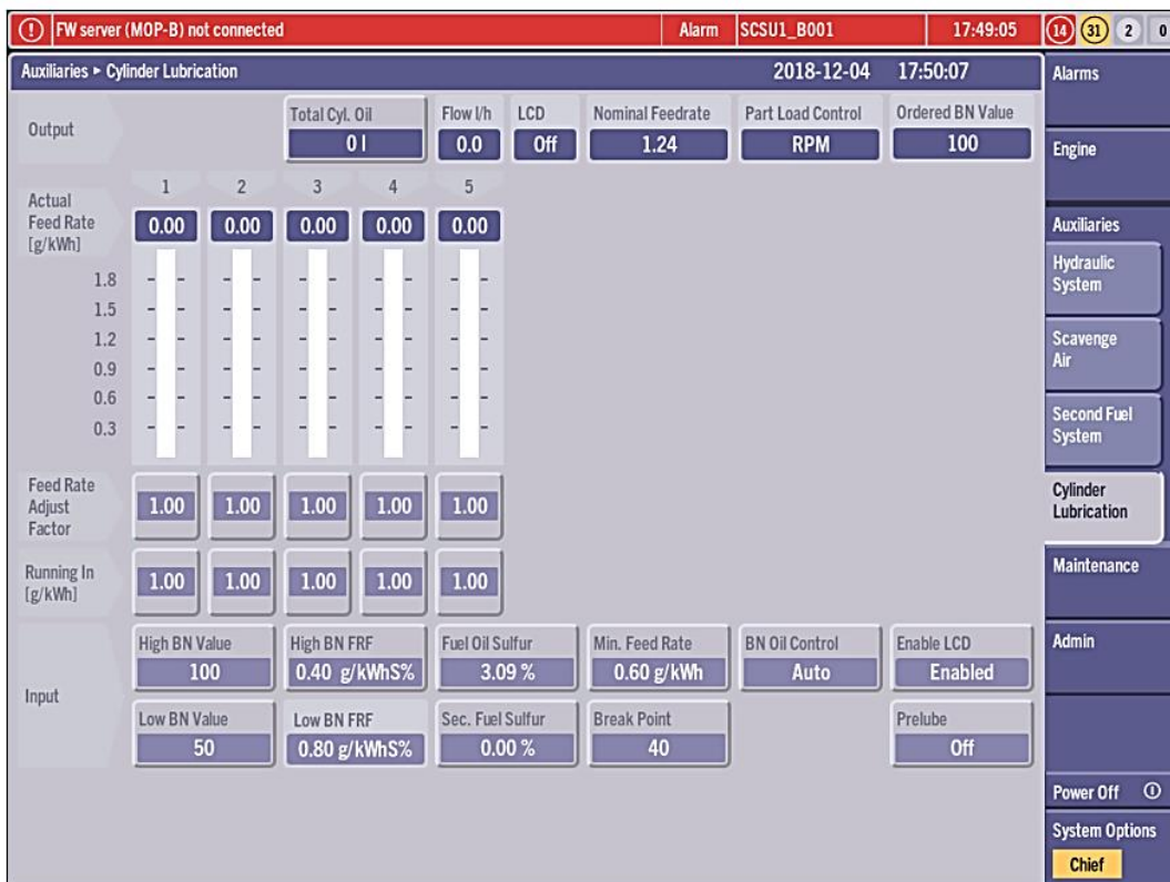
Fig. 12 ECS MOP Cylinder Lubrication page
