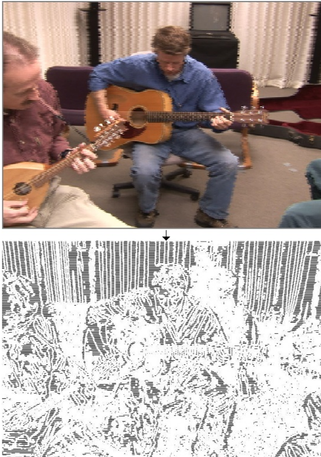
Figure 6. Detection of interlace artifact – gray pixels indicate distortion detection
