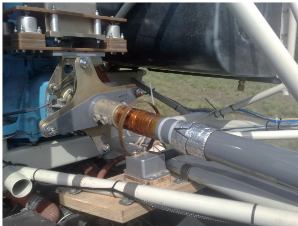
Fig. 4. Localization of torque meter with circular aerial on input shaft of main gear [J. Stanisławski, 2014]
