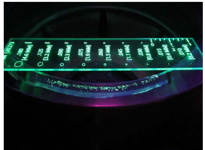
Fig. 2. The example of unconformity (porosity cluster) on the turbine outlet nozzle.
