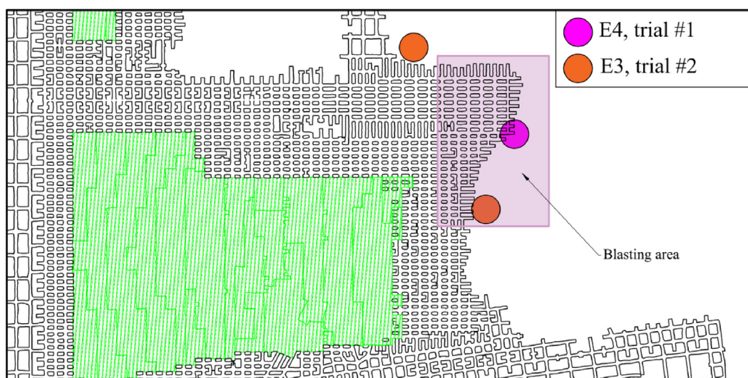
Fig. 13. Locations of the seismic events provoked by trials in panel B.
