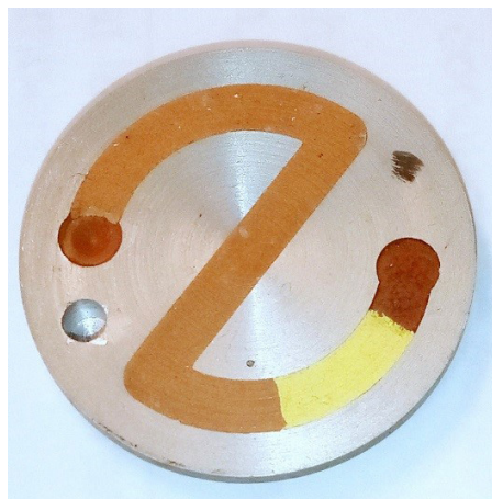
Figure 1. Unconfined (uncovered), curved, segmented pyrotechnic path pressed into the groove of the steel disc of a self-destructing timing assembly of an anti-aircraft short range missile
